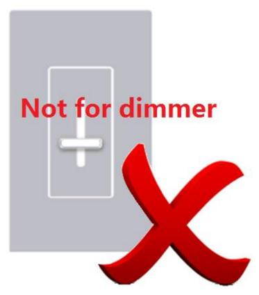
For dimming, LEEDARSON recommends using a compatible App (i.e., LEEDARSON'S LDS App) or a compatible wireless switch that uses the same wireless protocol as the bulb.
