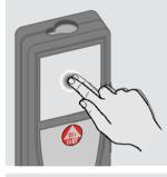
Tap on the display to open an onscreen button or to make a selection. Tapping on the icon in the mid of the bottom line activates the distance measurement or triggers the camera.
