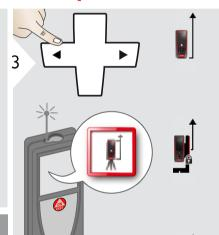
Distance is measured from the rear of the device (standard setting).
