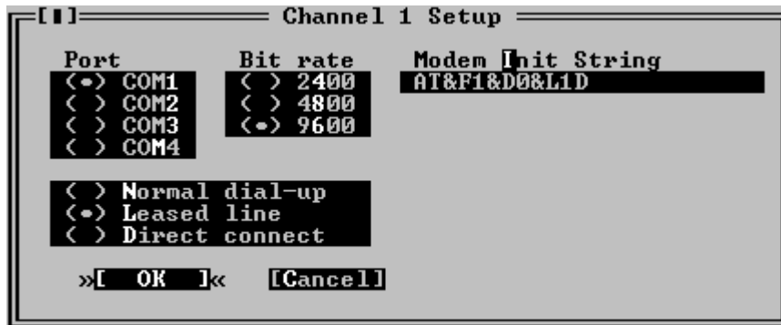
Figure 5-61 RMM channel setup for USR leased-line connections
