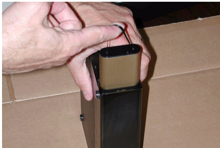
Figure 6-3: Removing Power/Transceiver Battery
