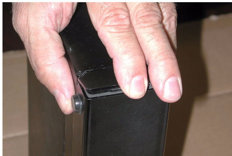
Figure 6-1: Loosening Power/Transceiver Battery Cover
