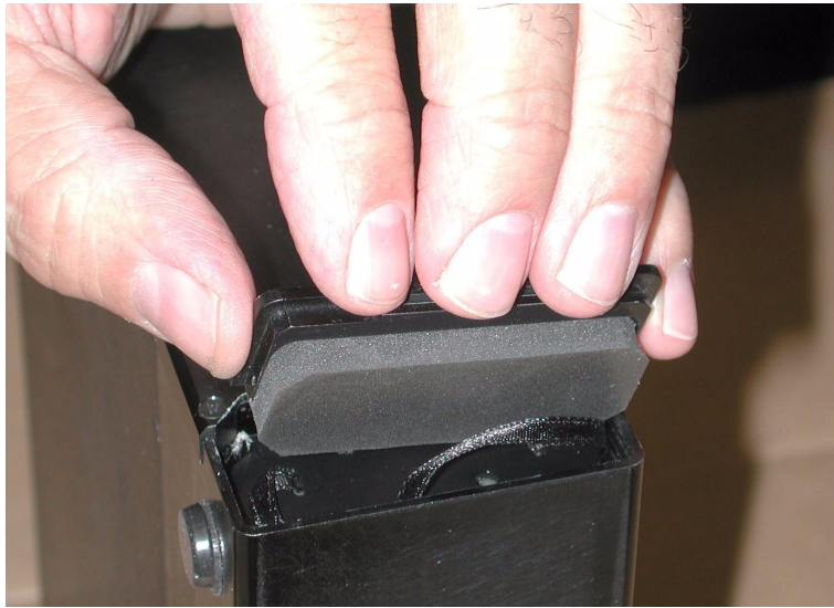
Figure 6-3: Removing Power/Transceiver Battery
