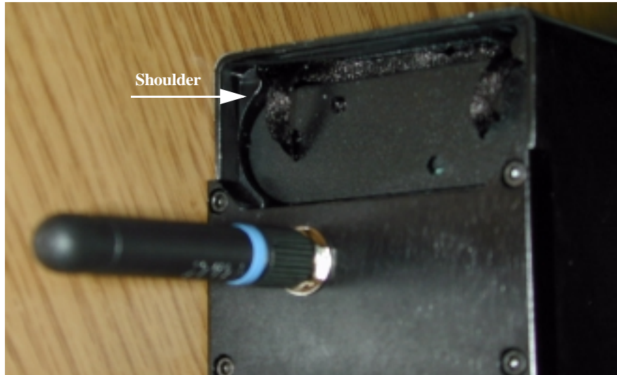
Figure 7-9. Wireless Imager Transceiver Battery Position Before Hatch Replacement
