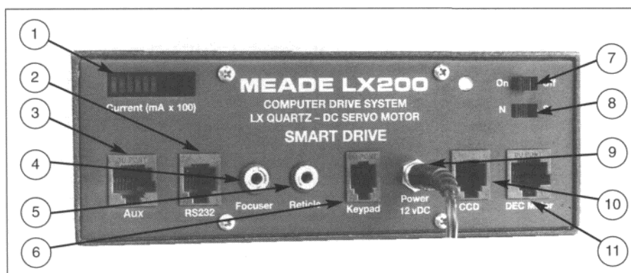
Fig. 7: 16" LX200 Power Panel. (1) Ammeter; (2) RS-232 Connector; (3) Aux Connector; (4) Focuser Connector; (5) Reticle Connector; (6) Keypad Connector; (7) ON/OFF Switch, (8) N/S Switch; (9) 12v DC Power Connector; (10) CCD Connector; (11) DEC Motor Connector.
