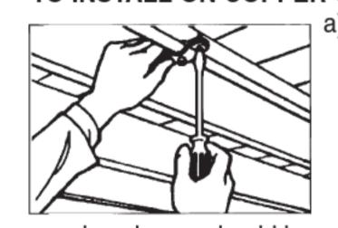
Place rubber gasket in center of hole in top saddle clamp. Place top and bottom saddle clamp around water pipe. Using bolts, tighten saddle clamps
