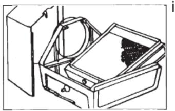
2. The unit is assembled for left side discharge. If right discharge is necessary, remove the right and left
