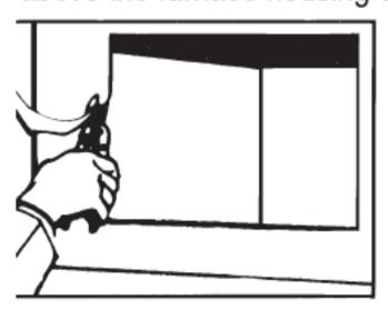
applicable), for clearance of the drain line. Trace around template edges. Remove the template and accurately cut the plenum opening 93/4"Wx121/2H, being careful to avoid injury from sharp edges.
