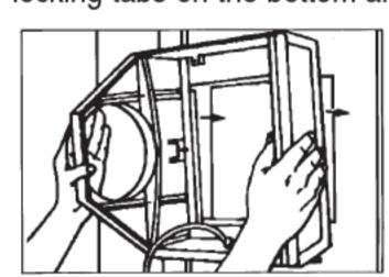
lower sheet metal edge. While holding the unit in place, install two screws at the top of the unit interior.
