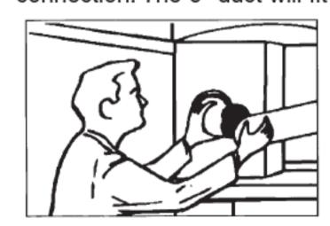
the side of the unit. If the system has central air conditioning, add a duct damper. Assemble components using sheet metal screws. Support bypass ducts in excess of 4' to prevent sagging.
