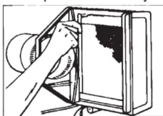
round receptacle at the bottom of the unit. Push the assembly in at the top against the beveled tabs. Replace the front cover.
