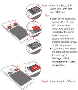
Only Micro SIM cards work with your smartphone. Always turn off your smartphone first before you insert or remove a Micro SIM card. Insert or remove a Micro SIM card with your smartphone on may damage your Micro SIM card or smartphone permanently.
