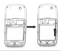
Warning: Make sure to power off the phone before taking out SIM card, otherwise your SIM card might be damaged.
