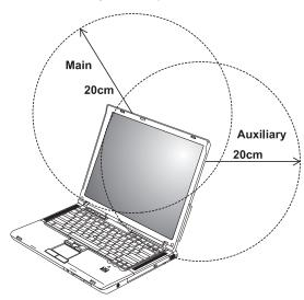
**Note:** The transmission diversity function is implemented for the models: WM3B2200BG, WM3B2915ABG, and AR5BMB-44. The function does not emit radio frequencies simultaneously from both antennas. One of the antennas is selected automatically or manually (by users) to have good quality of radiocommunication.
