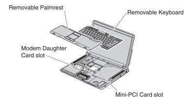
**Attention:** The ThinkPad Z60m Series computer contains an authentication mechanism You can install or remove each wireless feature by yourself. If you install an unauthorized wireless adapter that is not approved for use in the ThinkPad Z60m Series computer, the computer will not start, but only displays an error message and emits beeps.
