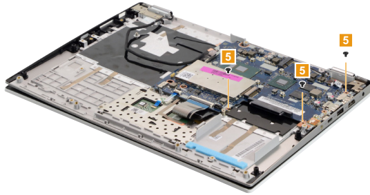
Figure 10. Removal steps of system board (continued)
