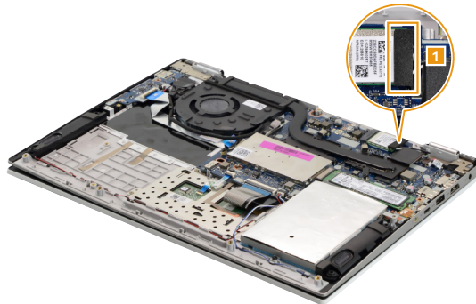
Figure 5. Removal steps of PCI Express Mini Card for wireless LAN
