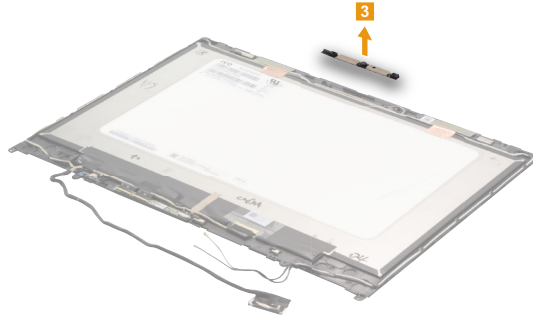
Figure 14. Removal steps of camera board, sensor board and EDP cable (continued)
