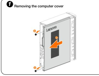
Replacing or upgrading hardware **①**
