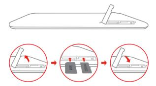
Step 1. Open the microSD card slot cover as shown.
