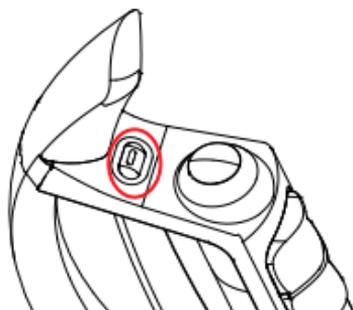
1. Press and hold the Power Switch for three seconds to turn on the controller.
