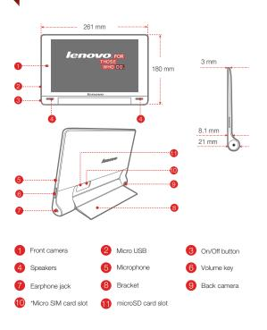
$\ensuremath{ @ \hspace{-8pt} }$  The WLAN model ( Lenovo B8080-F ) does not have a Micro SIM card slot.
