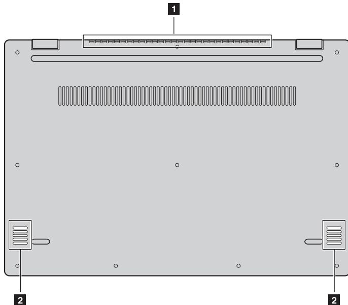
**1 Ventilation slots** Dissipate internal heat.
