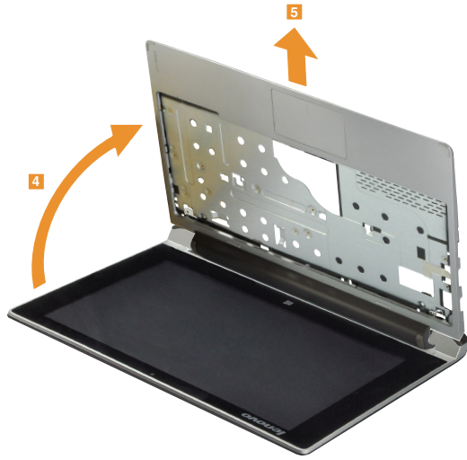
Figure 10. Removal steps of LCD unit (continued)
