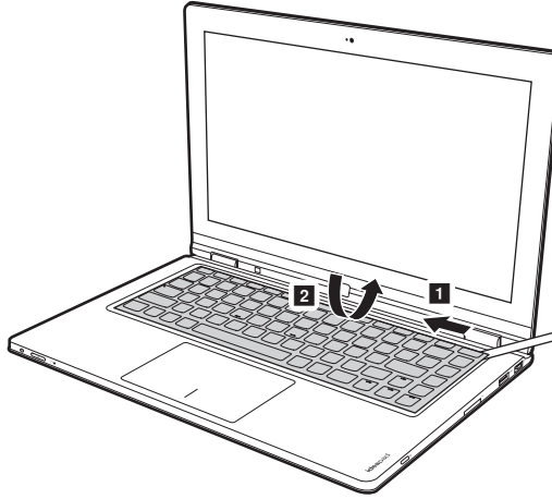
Figure 1. Removal steps of keyboard
