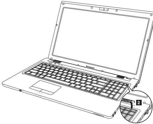
Figure 8. Removal steps of keyboard (continued)
