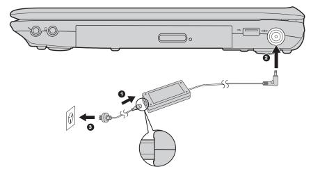
Connect the power cord to the AC adapter firmly, poor connections may result in damages to the AC adapter.
