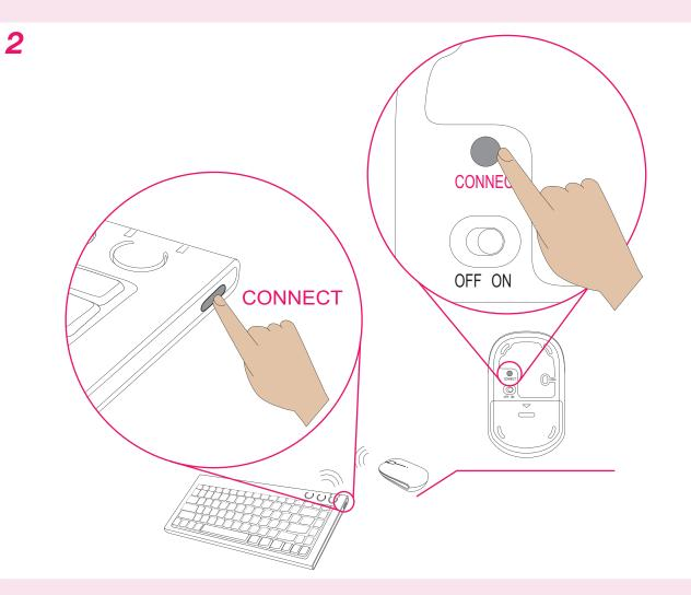
Press the wireless connect buttons on the right side of the keyboard and the back of the mouse for over 5 seconds.
