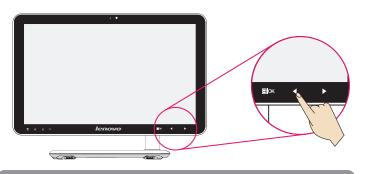
The buttons at the bottom of the screen are touch buttons. When you touch these, the indicator lights turn on.
