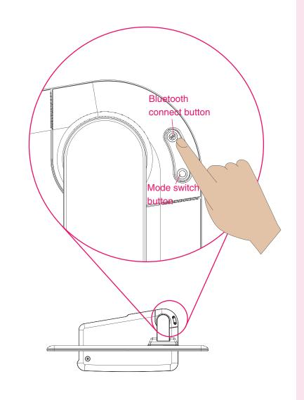
If connection is not established successfully, refer to "Wireless keyboard and mouse instructions" in the *User Guide*.
