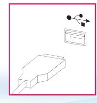
Connect the mouse cable to the appropriate mouse connector (USB connector).
