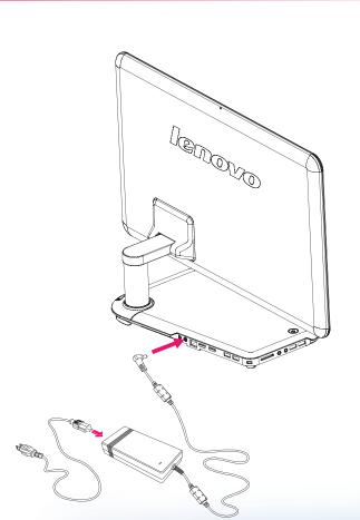
Connect the power cords properly to grounded electrical outlets.
