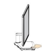
Press the power button on the top of the base stand to turn on the computer.
