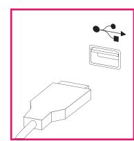
Connect the keyboard cable to the appropriate keyboard connector (USB connector).
