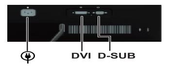
3. Connect one end of the analog signal cable to the monitor D-Sub connector and the other end to the computer.
