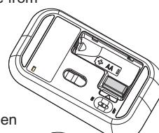
3. Insert one AA battery, then replace the battery cover.
