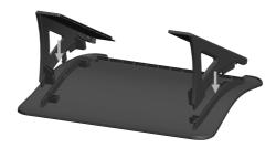
Step 2: Slide the removable panel (as indicated by the arrow) into the support structure. Audible sounds can be heard during the sliding process.
