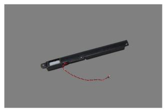
Figure 11-4. The removed right speaker
