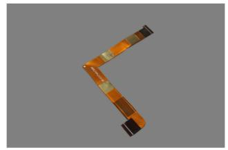
Figure 6-9. The removed LCD FPC
