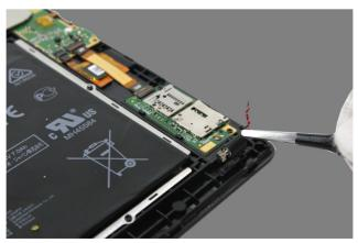
Figure 5-2. Removing the vibrator motor
