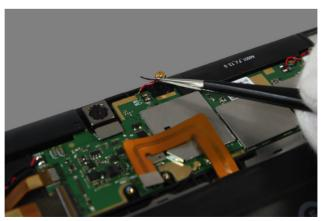
Figure 4-2. Removing the microphone
