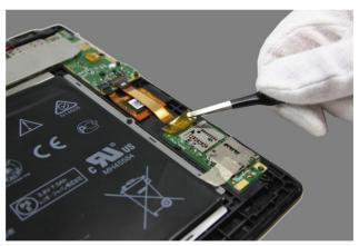
Figure 9-1. Removing the mylar on the main FPC (sub board side)
