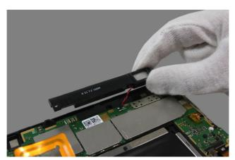
Figure 10-3. Removing the left speaker
