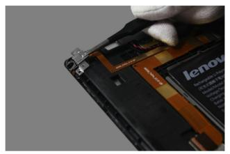
Figure 13-8. Removing the metal piece
