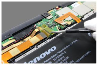
Figure 6-1. Removing the mylar on the LCD FPC (main board side)
