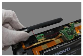
Figure 11-3. Removing the right speaker
