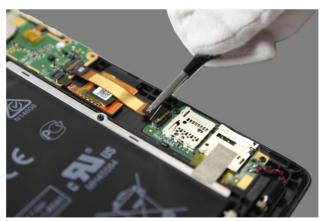
Figure 7-3. Pulling out the main FPC (from the sub board side)
