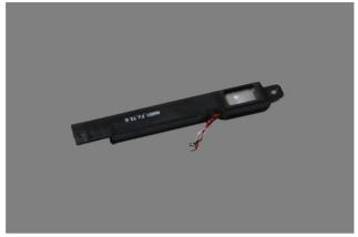
Figure 10-4. The removed left speaker
