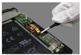
Figure 9-3. Pulling out the main FPC (from the sub board side)
