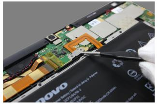
Figure 2-2. Removing the metal piece
