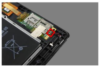
Figure 5-1. Position for desoldering the wires of the vibrator motor
