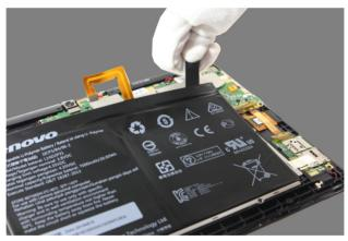
Figure 2-5. Detaching the battery pack
