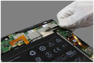
Figure 13-1. Peeling off the conductive fabric tape on the main board
