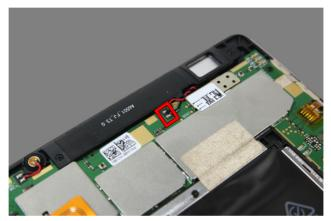
Figure 10-1. Position for desoldering the wires of the left speaker
