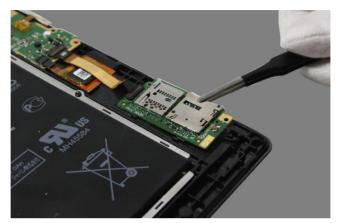
Figure 9-6. Removing the sub board
