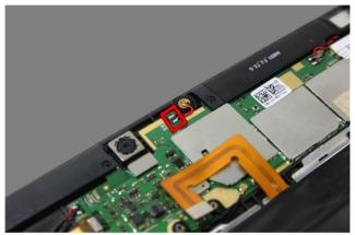
Figure 4-1. Position for desoldering the wires of the microphone
