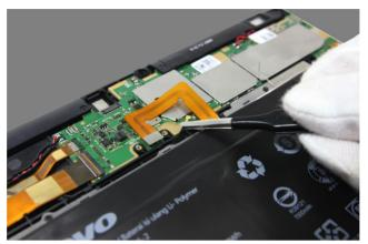
Figure 12-2. Positions for disconnecting the antenna cable (main board side, LTE version only)
