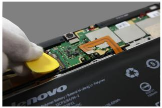
Figure 6-2. Unlocking the connector of the LCD FPC (main board side)
