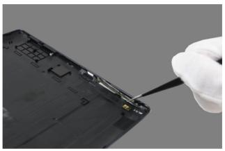
Figure 1-3. Removing the side key
