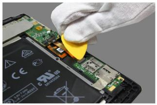
Figure 9-2. Unlocking the connector of the main FPC (sub board side)
