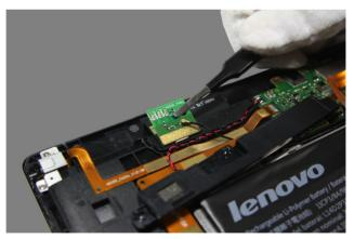
Figure 8-3. Removing the antenna PCB
