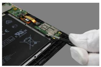
Figure 9-4. Removing the conductive fabric tape
