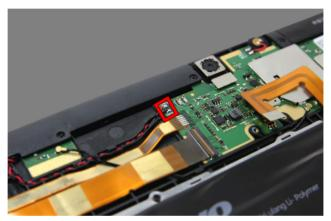
Figure 11-1. Position for desoldering the wires of the right speaker
