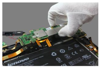
Figure 13-10. Removing the main board assembly from the front module of the tablet
