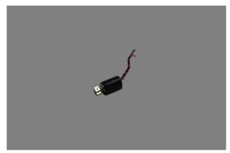
Figure 5-3. The removed vibrator motor
