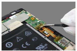
Figure 7-4. Removing the mylar on the main FPC (main board side)
