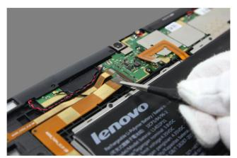
Figure 6-3. Pulling out the LCD FPC (from the main board side)
