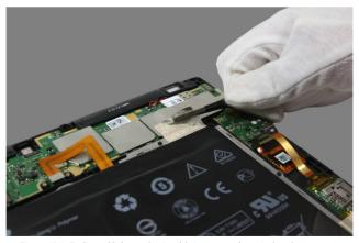
Figure 12-1. Peeling off the conductive fabric tape on the main board
