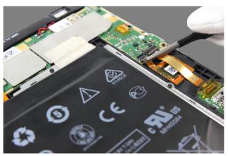
Figure 12-5. Pulling out the TP FPC
