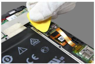
Figure 13-4. Unlocking the connector of the TP FPC
