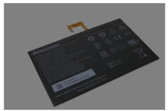
Figure 2-6. The removed battery pack
