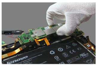
Figure 12-10. Removing the main board assembly from the front module of the tablet
