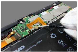
Figure 13-2. Positions for disconnecting the antenna cable (main board side, LTE version only)
