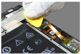
Figure 12-4. Unlocking the connector of the TP FPC
