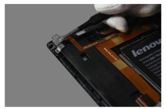
Figure 12-8. Removing the metal piece
