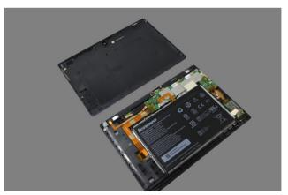
Figure 1-2. The removed rear cover with side key
