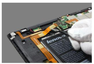
Figure 6-4. Detaching the LCD FPC
