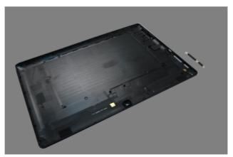
Figure 1-4. The removed rear cover and side key
