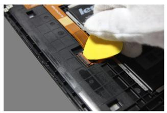
Figure 6-6. Unlocking the connector of the LCD FPC (front module side)
