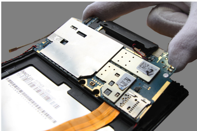
Figure 7-3. Detaching the main board assembly from the front module of the tablet
