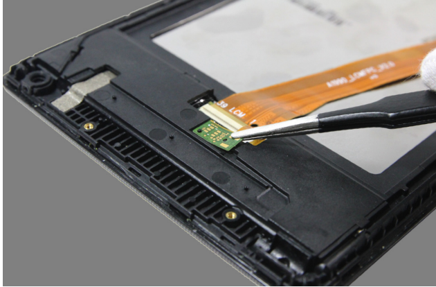
Figure 9-2. Detaching the main FPC PCB (Lenovo TAB 2 A7-30GC/H/HC/D/DC only)
