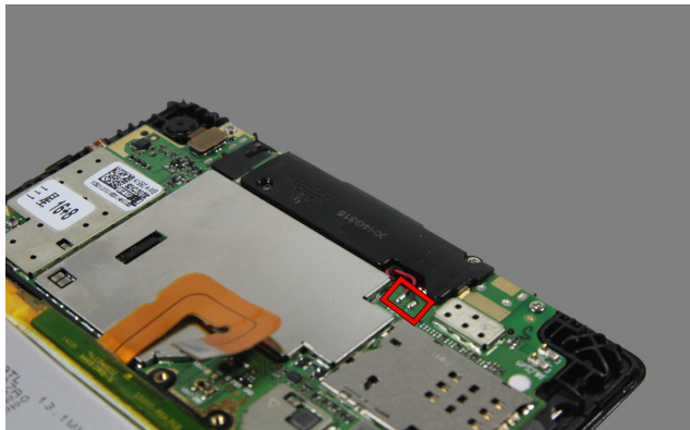
Figure 4-1. Position for desoldering the wires of the speaker (Lenovo TAB 2 A7-30GC/H/HC/D/DC)
