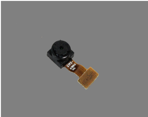
Figure 3-3. The removed rear camera
