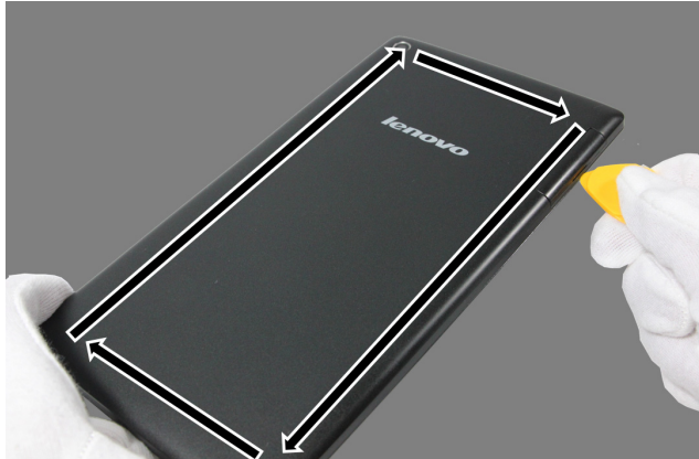
Figure 1-1. Unlocking the rear cover from the front module (along the joint line)
