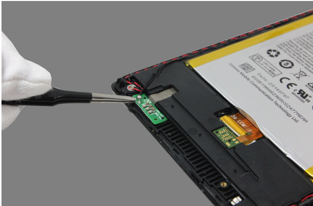
Figure 5-6. Detaching the antenna PCB (Lenovo TAB 2 A7-30GC)
