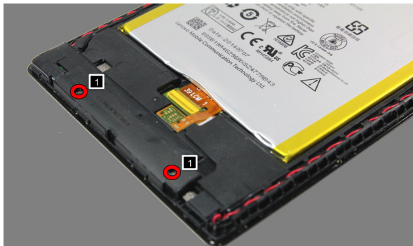
Figure 5-2. The screws on the antenna bracket (Lenovo TAB 2 A7-30H/HC/D/DC)
