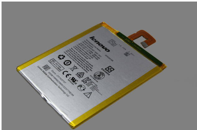
Figure 2-5. The removed battery pack
