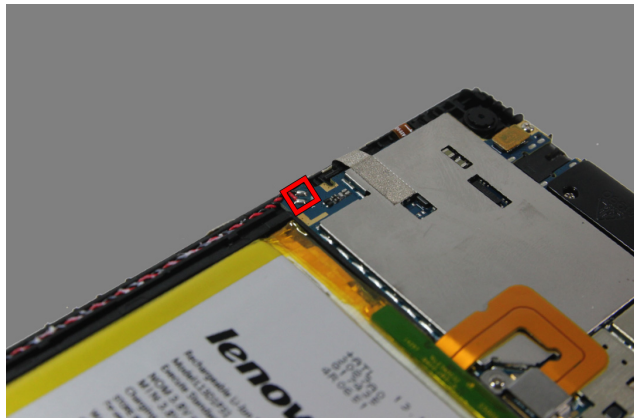
Figure 6-1. Position for desoldering the wires of the microphone
