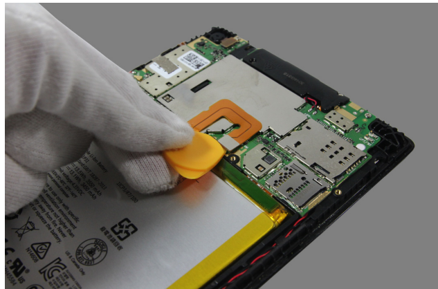
Figure 2-3. Disconnecting the battery FPC
