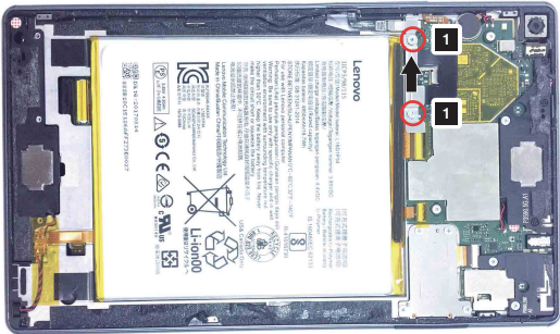
Figure 2. Removal steps of battery pack
