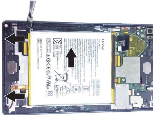
Figure 2. Removal steps of battery pack (continued)
