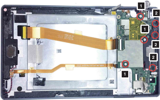
Figure 5. Removal steps of system board, speaker and microphone (continued) Remove the screws 1 and 2 .
