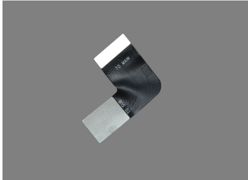
Figure 6-5. The removed main FPC
