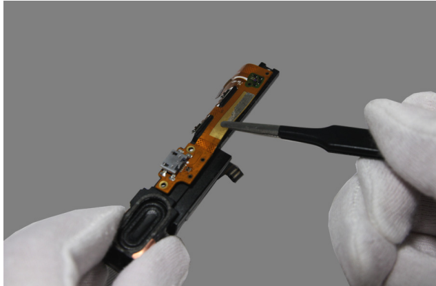
Figure 12-1. Detaching the USB and volume key FPC
