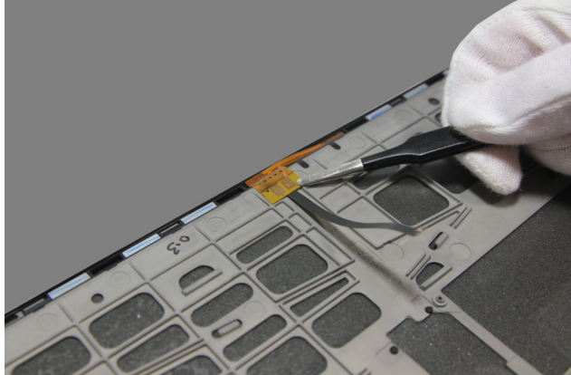
Figure 16-1. Detaching the WIFI2 antenna
