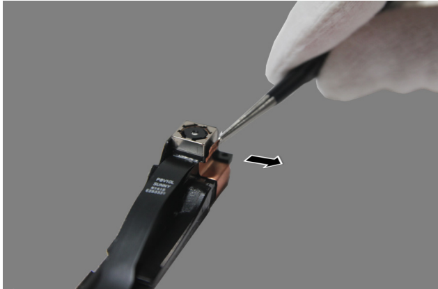
Figure 10-4. Detaching the conductive shield at the side of the rear camera
