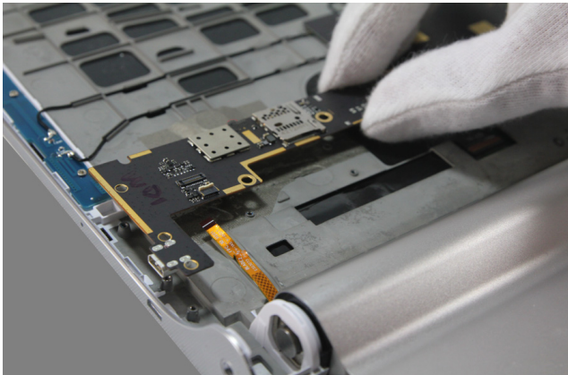
Figure 4-7. Removing the sub board
