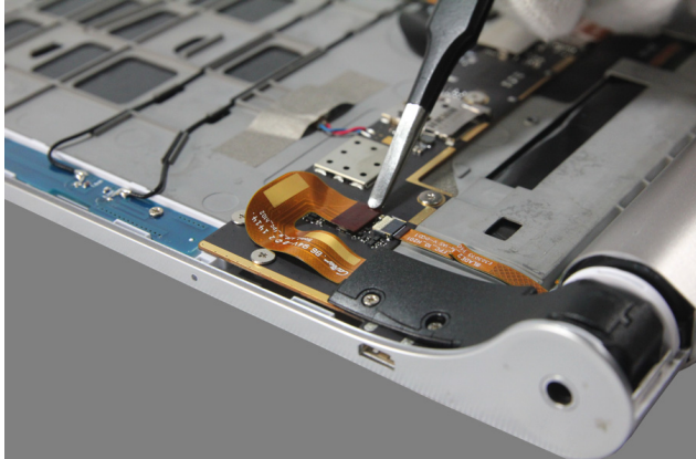
Figure 2-3. Detaching the FPC connector of the right speaker
