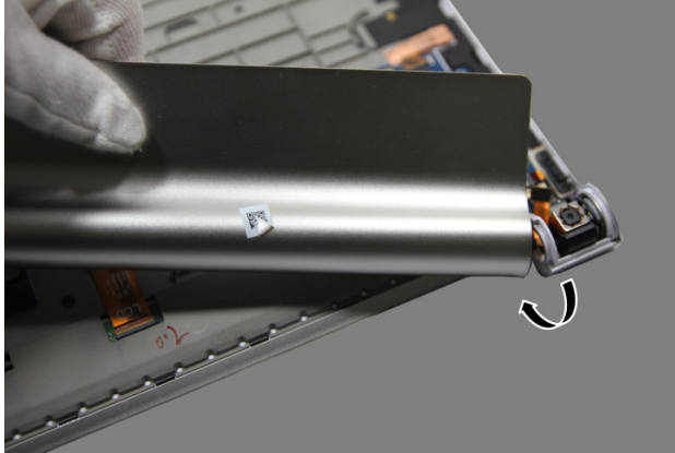
Figure 17-4. Removing the hinge frame with the battery pack
