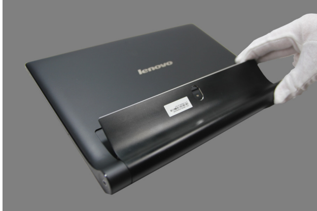
Figure 1-1. Opening the hinge frame
