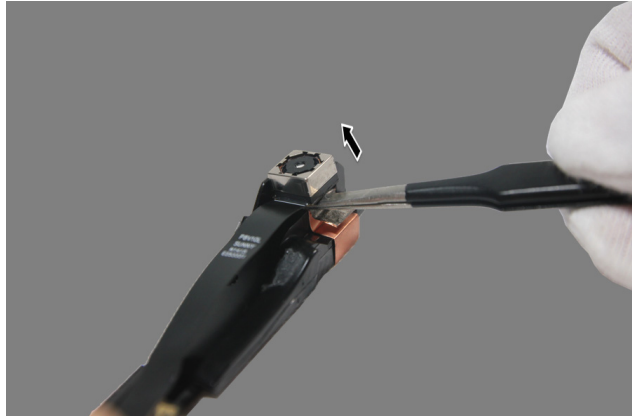
Figure 11-2. Removing the rear camera
