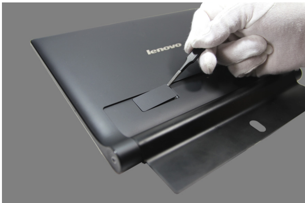
Figure 1-2. Opening the card slot
