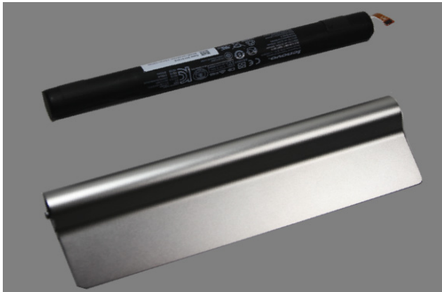
Figure 17-9. The removed battery pack
