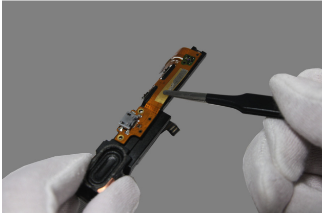
Figure 10-6. Removing the USB and volume key FPC
