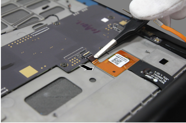
Figure 9-2. Pulling out the TP FPC
