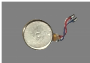
Figure 3-5. The removed vibrator motor
