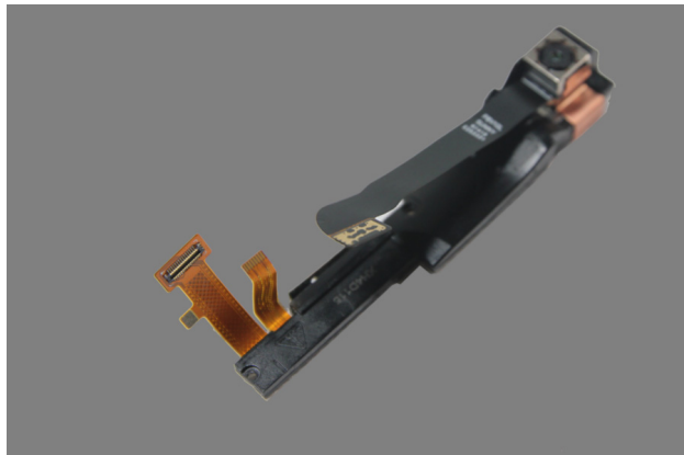
Figure 10-3. The removed left speaker together with attached rear camera and USB and volume key FPC
