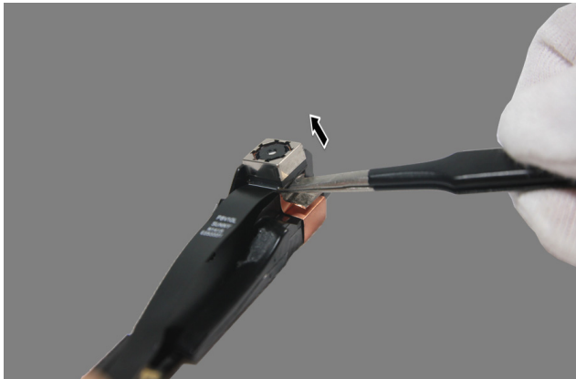
Figure 10-5. Removing the rear camera
