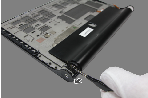
Figure 17-2. Pulling out the hinge pivot
