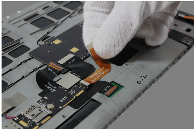
Figure 7-4. Removing the HDMI FPC
