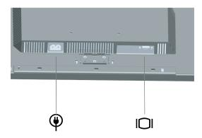
3. Connect one end of the analog signal cable to the monitor D-SUB connector and the other end to the computer.
