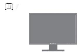
7. To optimize your monitor image, press the Automatic Image Setup key. Automatic image setup requires that the monitor is warmed up for at least 15 minutes. This is not required for normal operation.
