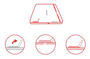
Open the card slot cover. Insert the Micro SIM card and the microSD card as shown. Close the card slot cover.
