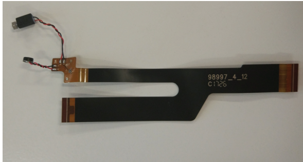
Figure 4. Removal steps of main FPC (continued)
