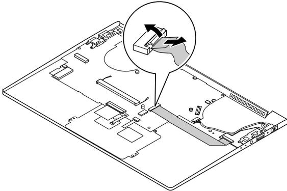
*Figure 22. Disconnect the cable*
