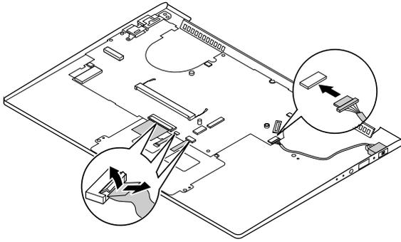
Figure 25. Disconnect the cable
