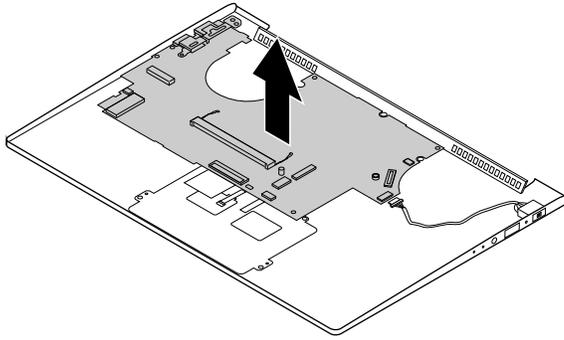
Figure 27. Remove the system board
