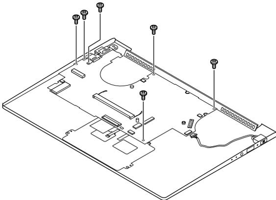
Figure 26. Remove 7 screws
