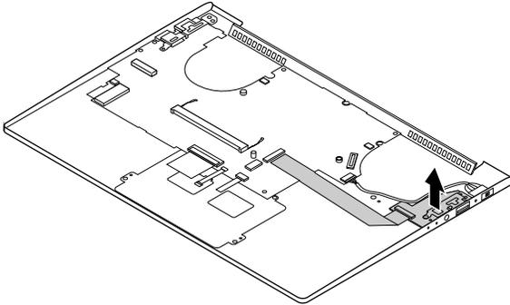
Figure 24. Remove I/O board and bracket
