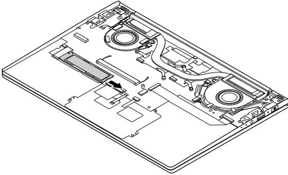
Figure 11. Remove by pulling the solid-state drive
