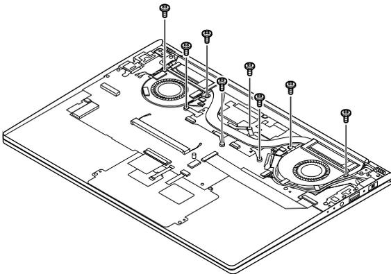
Figure 20. Remove screws
