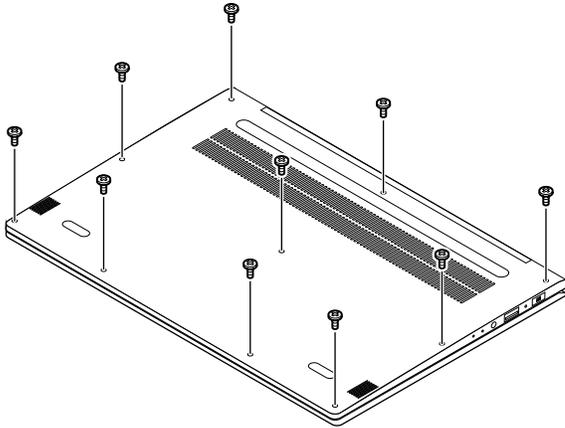
Figure 3. Remove 10 screws
