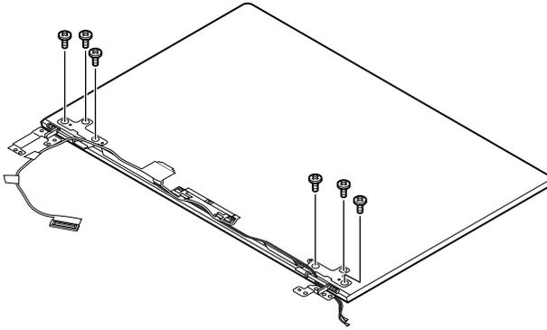
Figure 33. Remove 6 screws
