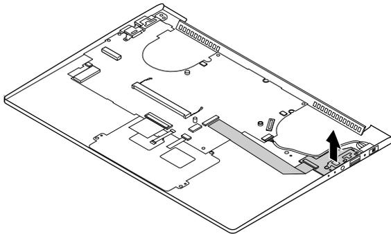
Figure 28. Remove I/O board and bracket
