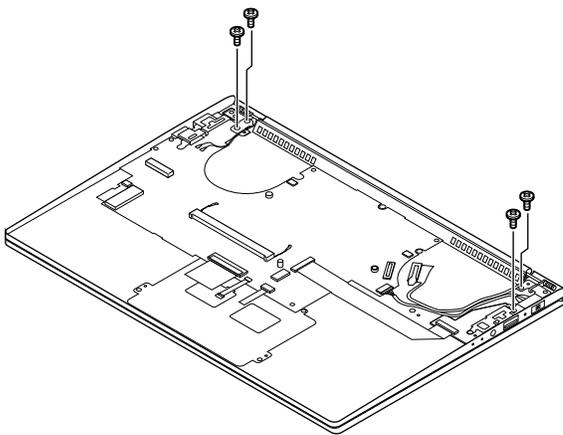
Figure 18. Remove 4 screws
