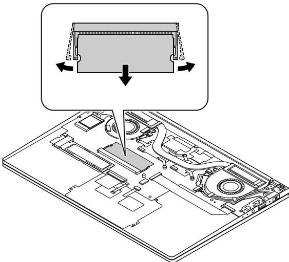
Figure 9. Remove the RAM module
