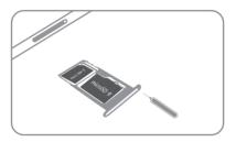
Insert the eject tool that comes with your smartphone into the hole in the card tray.
