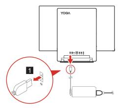
3. Remove the power cord from the power adapter.
