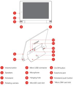
The WLAN model (Lenovo YT3-850F) does not have a Micro SIM card slot. You can use pencils or metal-tipped pens with a tip diameter of 0.7 mm or above, including fountain pens, rollerball pens, and some ballpoint pens, to write and draw on the screen or perform auxiliary touch operations. Special tip: There is a risk of scratching the screen slightly if you apply too much pressure when writing or use a pen tip that is too hard.
