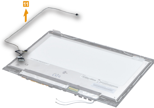
Figure 13. Removal steps of integrated camera, microphone board and cables (continued)
