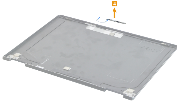
Figure 14. Removal steps of sensor board and camera board (continued)
