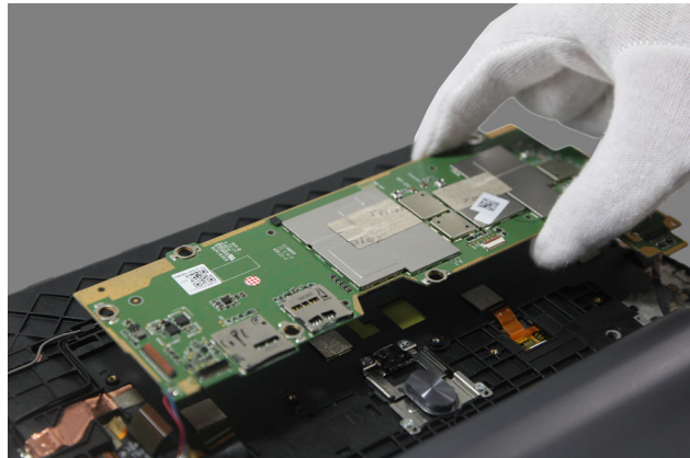
Figure 10-3. Removing the main board attached with vibrator motor
