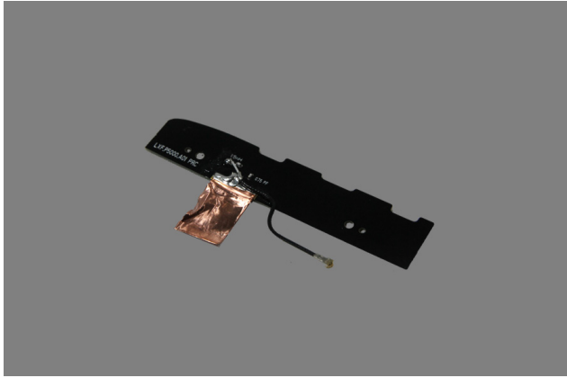
Figure 15-5. The removed antenna
