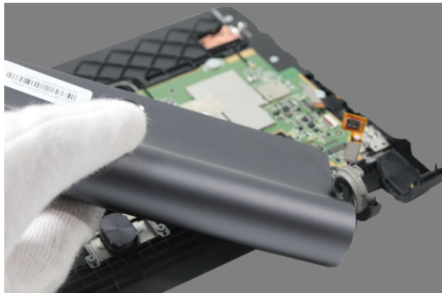
Figure 6-5. Removing the battery pack
