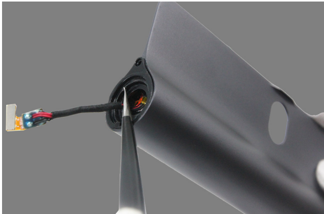
Figure 6-9. Removing the battery cover
