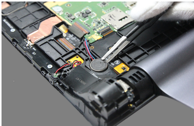
Figure 8-2. Detaching the vibrator motor
