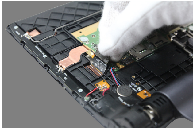
Figure 7-4. Removing the LCD FPC (from the front module side)
