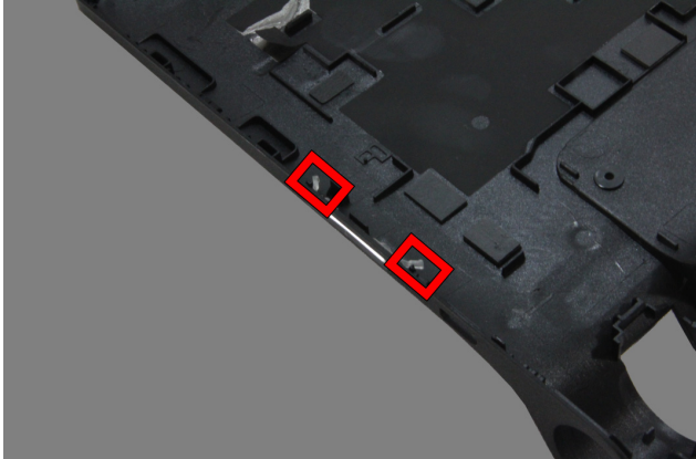
Figure 11-1. Detaching the volume key
