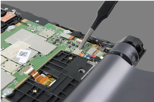
Figure 3-3. Disconnecting the power supply of the tablet
