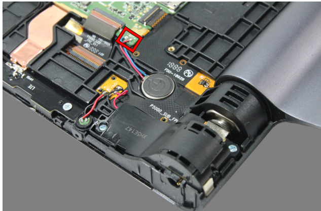
Figure 8-1. Position for desoldering the wires of the vibrator motor
