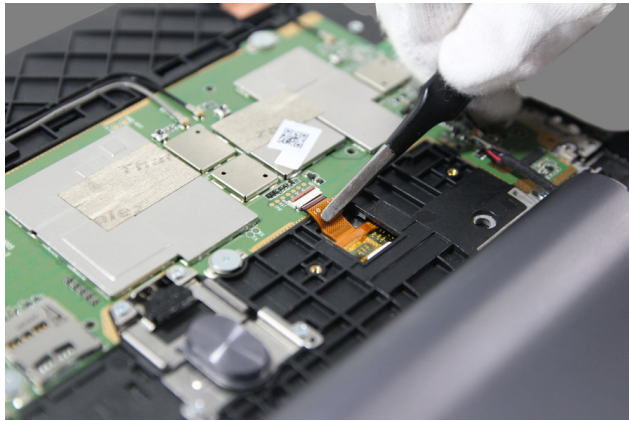
Figure 9-2. Pulling out the TP FPC
