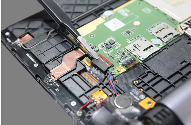
Figure 7-2. Pulling out the LCD FPC (from the main board side)
