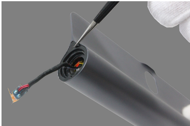
Figure 6-7. Peeling off the foil on the battery cover
