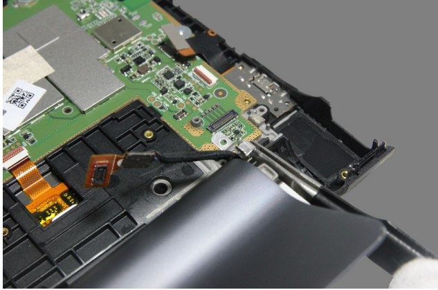
Figure 6-2. Removing the metal piece
