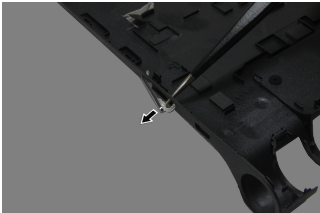
Figure 11-2. Removing the volume key
