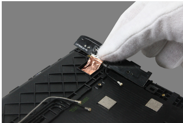
Figure 15-4. Removing the antenna
