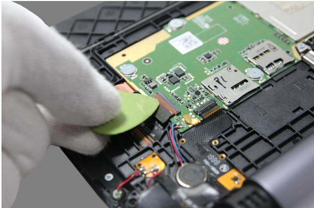
Figure 7-1. Unlocking the connector of the LCD FPC (main board side)
