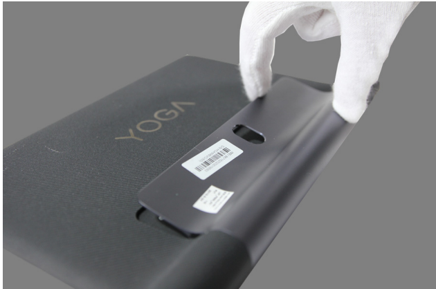
Figure 1-1. Opening the hinge frame
