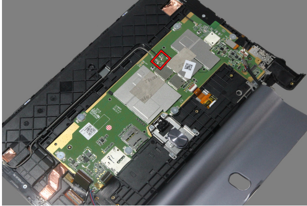
Figure 13-2. Positions for disconnecting the antennas
