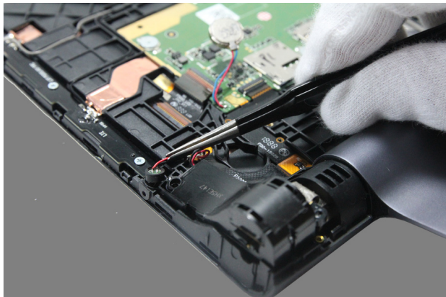
Figure 5-3. Detaching the microphone
