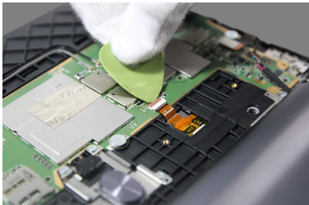
Figure 9-1. Unlocking the connector of the TP FPC
