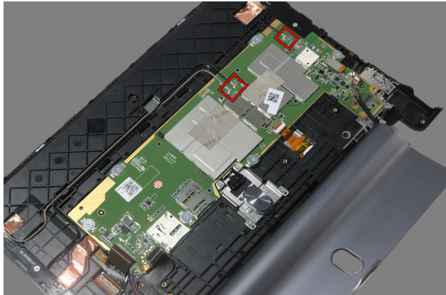
Figure 9-4. Positions for disconnecting the antennas
