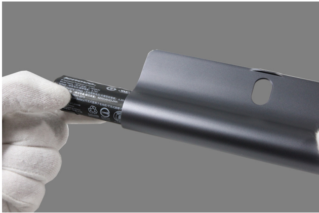
Figure 6-10. Removing the battery cell
