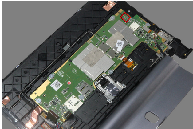
Figure 14-1. Positions for disconnecting the antennas
