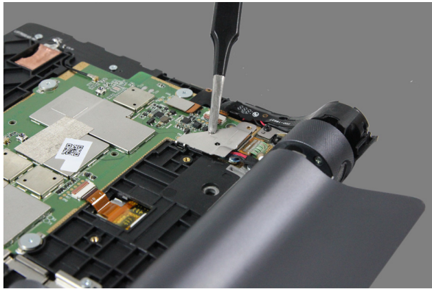
Figure 3-2. Removing the metal piece
