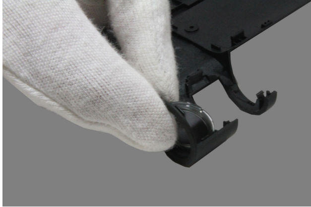
Figure 12-1. Removing the power button
