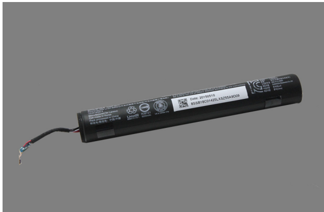
Figure 6-11. The removed battery cell
