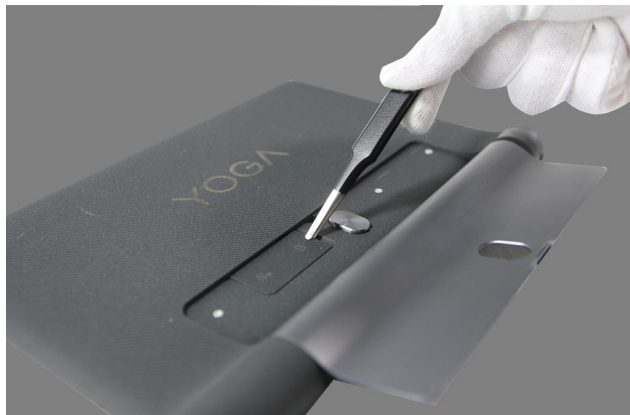
Figure 1-2. Removing the card slot cover
