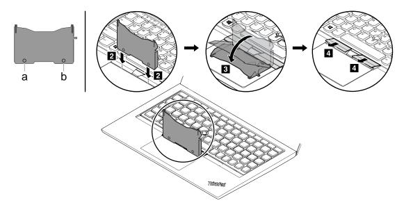
3. Loosen the screws that secure the keyboard with screw torque 0.143Nm (1.4kgf-cm).
