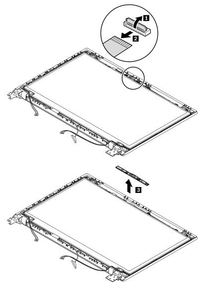
Removal steps of the camera/microphone combo card - for models with traditional camera
