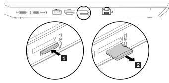
After you finish the service, insert the card back into the slot.
