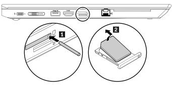
After you finish the service, install the tray and the card back into the slot.
