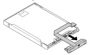
Removal steps of the 2.5-inch internal-storage-drive bracket
