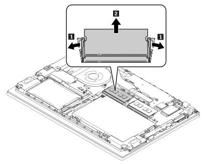
**When installing:** Insert the notched end of the memory module into the memory slot at an angle of about 20 degrees. Press the memory module in firmly, and pivot it downward until it snaps into place. Ensure that the memory module is firmly installed and does not move easily.
