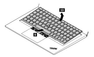
8. Put the keyboard on the palm rest as shown. Open the plastic shield and detach the connectors. Then remove the keyboard.
