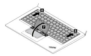
6. Pivot the tool in the direction as show to release the keyboard **1**. Push the keyboard in the direction as shown by arrows **3** to release the latches from the keyboard bezel.
