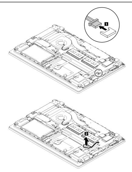
When installing: Ensure that the connector is firmly attached.
