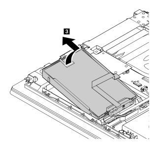
Removal steps of the 2.5-inch internal-storage-drive cable
