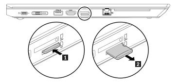
After you finish the service, insert the cards back into the slot.
