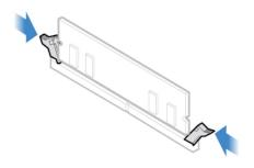
Figure 26. Securing a memory module with the latches
