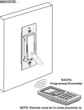
NOTE: Remote must be in close proximity to dimmer when including in the network.
