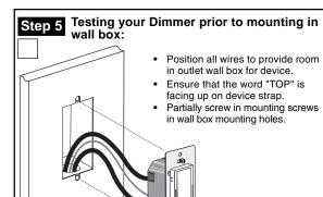
NOTE: Dress wires with a bend as shown in diagram in order to relieve stress when mounting device.
