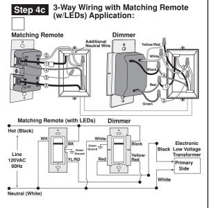
**NOTE:** The dimmer **must** be installed in a wall box that has a Load connection. The matching remote must be installed in a wall box with a Line Hot connection and a Neutral connection. A Neutral wire to the matching remote needs to be added as shown. If you are unsure about any part of these instructions, consult a
