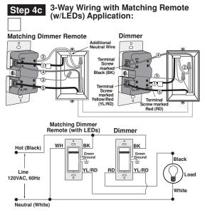
**NOTE:** The dimmer **must** be installed in a wall box that has a Load connection. The matching remote **must** be installed in a wall box with a Line Hot connection and a Neutral connection. A Neutral wire to the matching remote needs to be added as shown. If you are unsure about any part of these instructions, consult a
