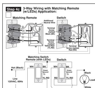
NOTE: The switch must be installed in a wall box that has a Load connection. The matching remote must be installed in a wall box with a Line Hot connection and a Neutral connection. A Neutral wire to the matching remote needs to be added as shown.
