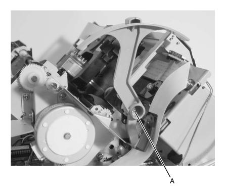
Remove the screw [A] securing the carrier motor bracket to the bottom cover.
