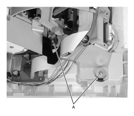
5. Remove the two grommet anchored screws [A] from the right side of the print unit.
