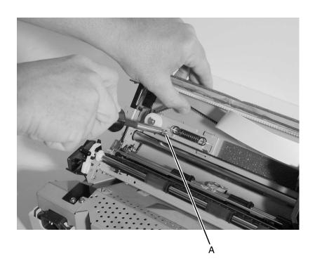
4. Remove the retaining wire [A] from the left side of the carrier shaft.
