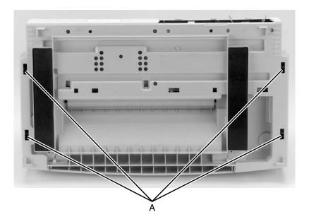
10. Turn the printer right side up and insert a flat blade screwdriver into each of the two holes [A] in the back of the top cover.
