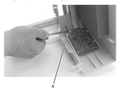
4. While holding the latches down, push the operator panel out of the top cover, toward the bottom of the cover.
