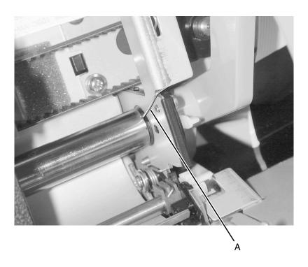
5. Remove the screw [A] from the forms thickness lever and remove the lever.
