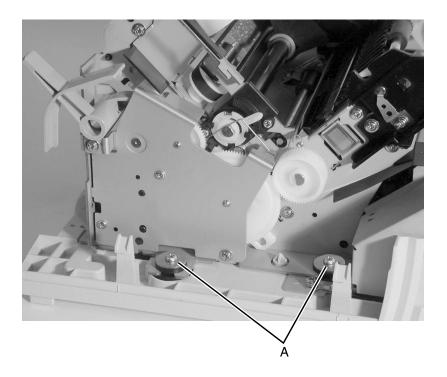
6. Remove the print unit from the bottom cover, by pulling up forcefully on both sides of the print unit.
