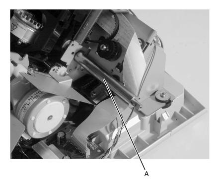
10. Remove the carrier from the printer.
