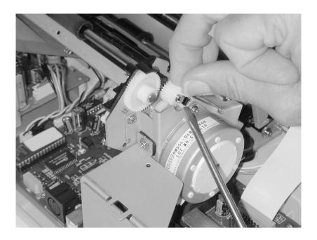
4. Remove the two screws [A] from the right upper feed roller bracket. One screw also retains the upper feed roller ground clip.
