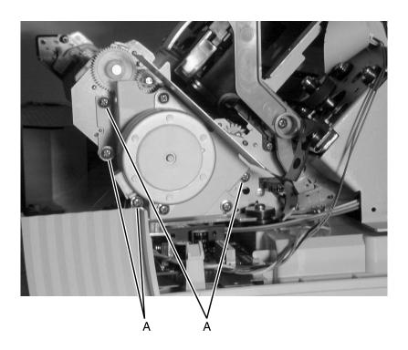
4. Remove the paper feed motor bracket assembly, exposing the gears, as shown.
