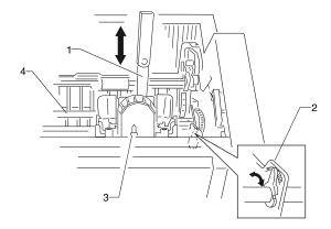
10. After adjusting both left and right gap adjust bushings, push the printhead to the center of the platen and verify a gap of within (0.33 and 0.37 mm) exists between the printhead and the platen.
