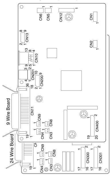
Logic Board - Printhead (9w)
