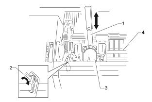
9. Move the printhead to the right edge of the rubber on the platen and using a feeler gauge [1], slowly adjust the right gap adjust bushing [2] clockwise, until a gap of (within 0.33 and 0.37 mm) exists between the printhead [3] and the platen.
