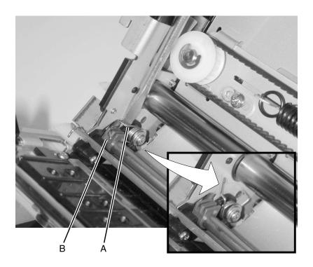
8. Slide the carrier to the right side of the printer.
