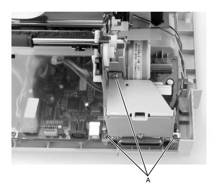
3. Remove the four screws [A] from the paper feed motor bracket assembly.
