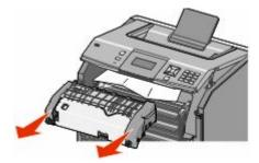
c Place the fuser unit on a flat surface.
