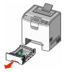
Notice the size indicators on the bottom of the tray. Use these indicators to help position the guides.
