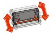
**9** Remove the red packing strips from the new cartridge.
