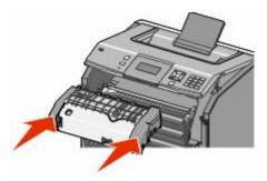
**5** Turn the screws to the right to securely fasten the fuser unit.
