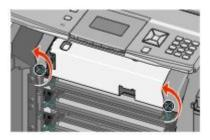
2 Lift the handholds on each side of the fuser unit, and then pull forward to remove it.
