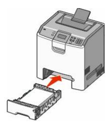
**7** If a different type of paper was loaded than the type previously loaded in the tray, then change the paper type setting for the tray from the printer control panel. For more information, see "Setting the paper size and type" on page 55.
