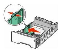
Notice the load line on the left side of the paper tray: it indicates the maximum height for loading paper.
