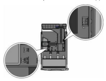
**2** Squeeze the width guide tabs as shown, and then slide the guide to the correct position for the size of paper being loaded.
