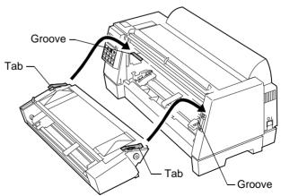
**5** Attach the front paper supports to the Auto Sheet Feeder.
