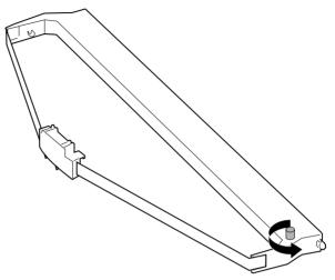
Manually move the ribbon guide to the far side of the cartridge, as shown below, then rotate the ribbon advance knob to take up any slack in the ribbon.
