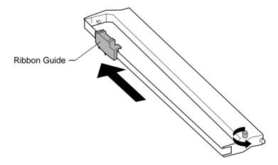
**6** Insert the ribbon guide over the metal pins on each side of the printhead.
