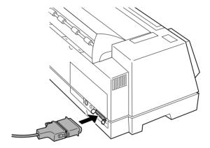
If you do not wish to use our recommended DB 25 to DB 25 null modem cables, or if you already have a similar RS 232 null modem cable, you may only need to attach Lexmark's DB 25 to Centronics 36 Serial Adapter (part number 1319143) to your existing cable.
