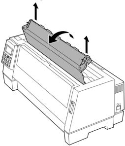
**3** Carefully pull up on the ribbon guide while also pulling up on the ribbon cartridge. The cartridge unlatches from the printer.
