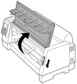
**6** Pull up the left and right tractor locking levers to unlock the tractors.
