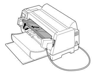
**7** Pull up the left and right tractor locking levers to unlock the tractors.
