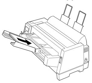
**7** Move the paper guide so the print start position you want aligns with the symbol [A printed on the margin guide of the Auto Sheet Feeder.
