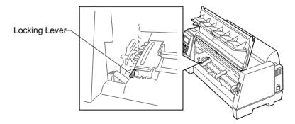
Move the left tractor to the left or right of the [A symbol. Push down the left tractor locking lever to lock it in place. Remove slack from the paper and lock the right lever.
