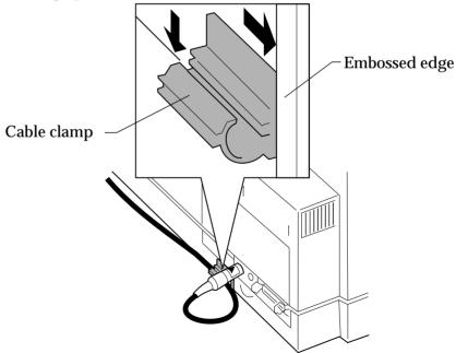
**13** Insert the Tractor 2 Feeder cable into the clamp, as shown, and snap the clamp shut.
