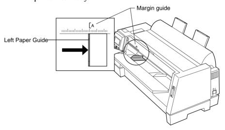
**6** Place a single sheet against the left paper guide. Move the right paper guide so that the guide aligns with the right edge of the paper.
