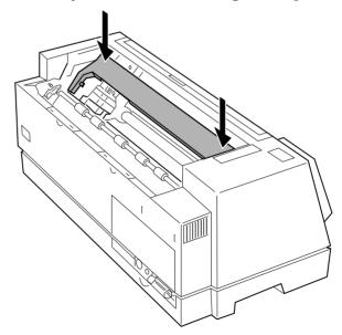
**9** Make sure the ribbon feeds smoothly by rotating the ribbon advance knob counterclockwise.
