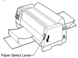
**3** To clear the paper path, tear off the leading edge of the continuous form, as shown.
