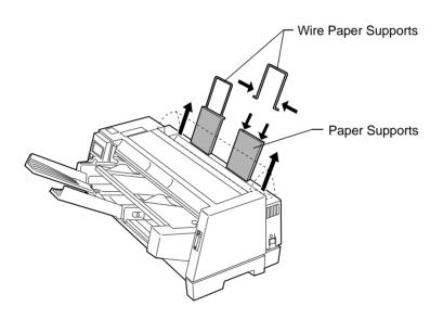
**7** Attach the front cover that came with the Auto Sheet Feeder.
