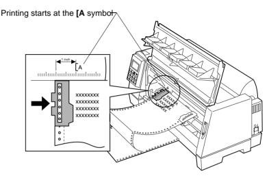
The distance from the **[A** symbol to the left edge of the paper determines the width of the left margin.
