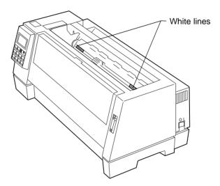
**Note:** When the ribbon cartridge is installed and the top edge of the paper is even with the top edge of the ribbon, the TOF is set to one line, or 1/6 inch.
