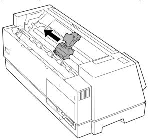
**4** Rotate the ribbon advance knob on the ribbon cartridge counterclockwise to ensure that the ribbon feeds smoothly. If necessary, untwist the ribbon.
