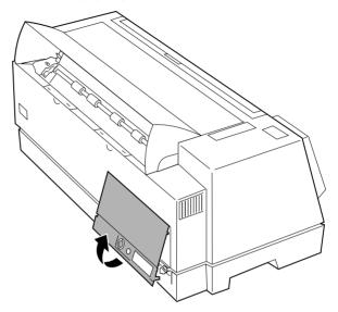
On the system board cover, twist the knockout plug to remove it.
