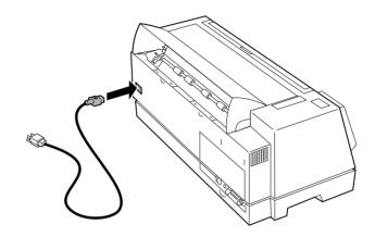
**3** Connect the other end of the power cord to a properly grounded electrical outlet.
