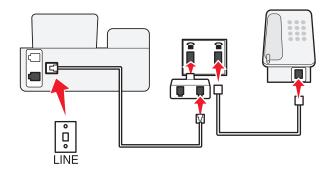
If the additional device (telephone or answering machine) has an RJ-11 connector, then you can remove the wrap plug and plug the device into the 🗐 port of the printer.
