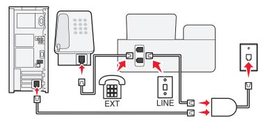
A Digital Subscriber Line splits your regular telephone line into two channels: voice and Internet. Telephone and fax signals travel through the voice channel, and Internet signals pass through the other channel. This way, you can use the same line for analog voice calls (including faxing) and digital Internet access.
