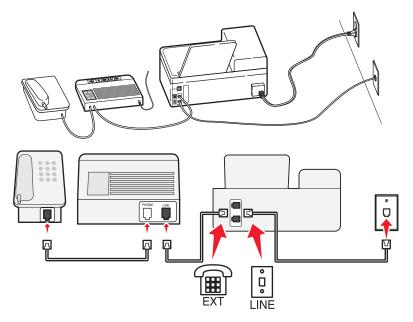
**Connected to different wall jacks**
