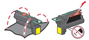
7 Insert the new cartridge into the printer, and then push the green handle back in place.Note: Make sure the cartridge is fully pushed in.
