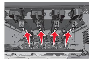
4 Clean the lenses using compressed air.
