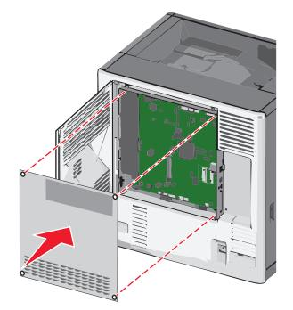
**b** Align and then turn each screw clockwise to tighten.
