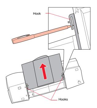
**6** Pull the paper exit tray all the way out of the printer.
