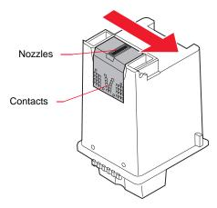
To dissolve dried ink, hold the damp cloth against the nozzles for about three seconds. Gently blot and wipe dry.
