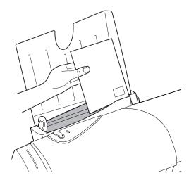
**3** *Squeeze* the release tab and the paper guide together, and slide the paper guide to the right until it rests against the envelopes or card stock.
