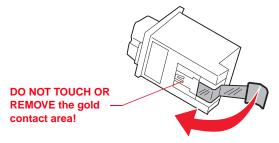
2 Insert the replacement print cartridge in the print cartridge carrier.
