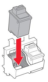
**3** Push back firmly on the cartridge until it *snaps* securely into place.
