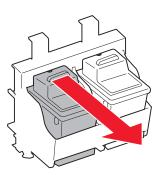
**5** Remove the print cartridge by lifting it straight out of the printer.
